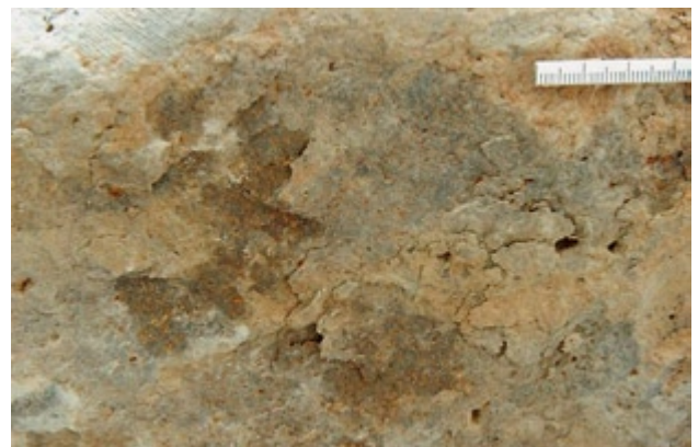
Fig. 2 Detailed view of the weathered crust on a stone: it has already been lost in the darker regions to the left; there are several loose particles on the right. © VG BILD-KUNST Bonn, 2006. © Bayerische Staatsgemäldesammlungen, Munich. Photo: S. Forster.
